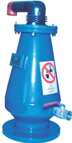
SPS air release valve incorporates a kinetic and an automatic air release valve in one single valve body. Each function in the sewage system is to release air (gases) and to admit air into sewage and waste water lines. The exclusive structure guarantees complete separation of the liquid from the sealing system and provides optimum working conditions.
